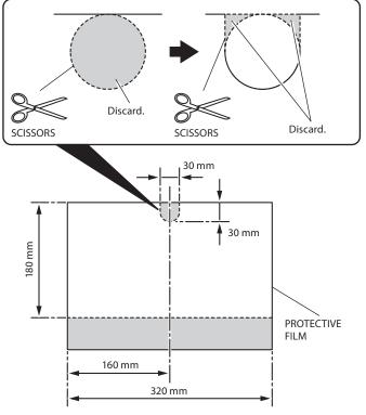
3 Attach the protective film on the rear fender as shown.
