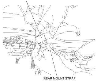
6. Insert both left and right rear strap buckles into their mating parts attached to the rear of the bag.
