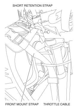
8. Route the free end of the front mount strap under the steering head of the bike and up behind both the clutch cable and electric wiring harness. Make sure the strap stays in front of the steering stop rod.
