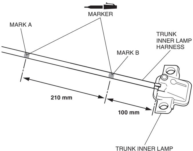
4. Install the trunk inner lamp as shown.
