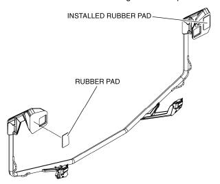
Install two Honda Pro-Connect<sup>™</sup> latches into the front carrier extender using a rubber spacer between each latch and the carrier extender. Secure the latches to the front carrier extender by installing a snap ring onto each latch from underneath the carrier extender.
