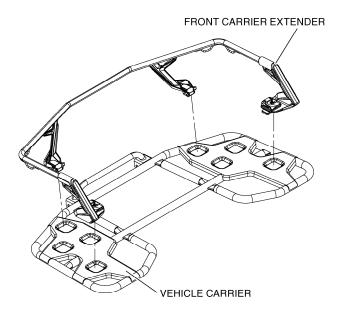
4. Secure the front carrier extender to the vehicle carrier by pressing down each Honda Pro-Connect  $^{\!\top\!M}$  lever.
