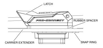
3. Lift the lever on each latch to unlock them. Place the front carrier extender onto the front carrier of the ATV. Line up each latch with its corresponding hole in the carrier then push each latch into its hole.
