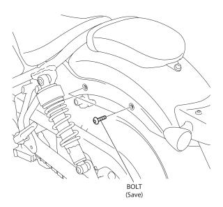
2. Loosely install the rear carrier as shown.
