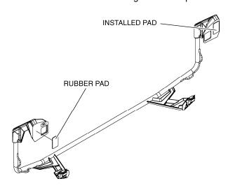
2. Install two Honda Pro-Connect<sup>™</sup> latches into the rear carrier extender using a rubber spacer between each latch and the carrier extender. Secure the latches to the rear carrier extender by installing a snap ring onto each latch from underneath the carrier extender.
