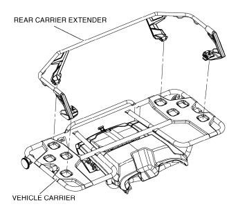
4. Secure the rear carrier extender to the vehicle carrier by pressing down each Honda Pro-Connect<sup>™</sup> lever.
